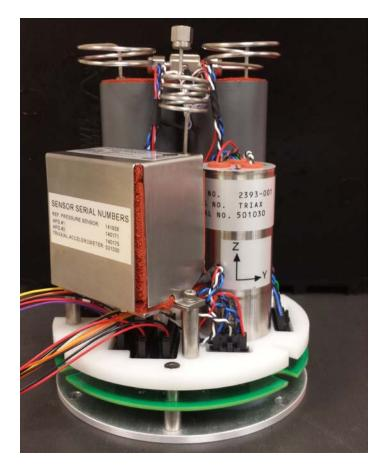
Temperature compensated and linearized RS-232 outputs are provided from all sensors:
