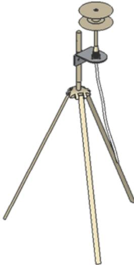
Figure 5. Digiport mounted on a mast
