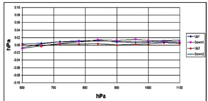
Figure 5. Barometer Repeatability, Hysteresis and Linearity
