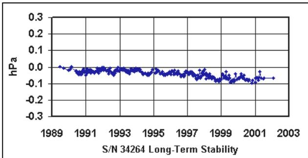
Figure 6. 12-Year Barometer Stability Test
