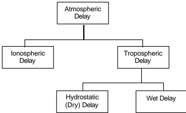
Figure 1. Causes of Atmospheric Delay
