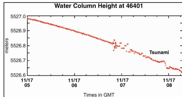
**Figure 8. Tsunami of November 17, 2003 as measured at the tsunameter located at 50°N 171°W in 4700 m water depth.**
