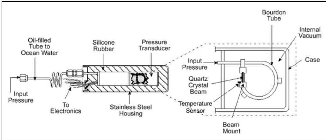
Figure 3. Digiquartz® Bourdon Tube Broadband Depth Sensor
