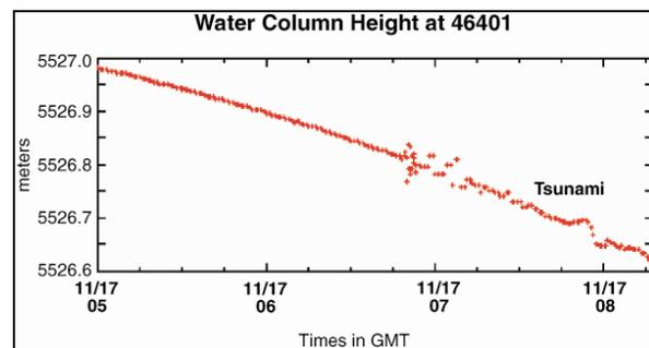
**Figure 8. Tsunami of November 17, 2003 as measured at the tsunameter located at 50°N 171°W in 4700 m water depth.**
