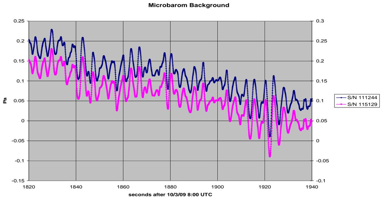
Fig. 6: Typical microbarom background from Fig. 4 just before the volcano sound wave arrived. Sensor 2 (in red) is visually offset by 50 mPa (right vertical axis) to show how well it tracks Sensor 1 (in blue). The amplitudes of the microbaroms vary daily and seasonally. Here they were about 0.1 Pa peak-to-peak (1 microbar – hence the name) with a period of about 5 seconds.
