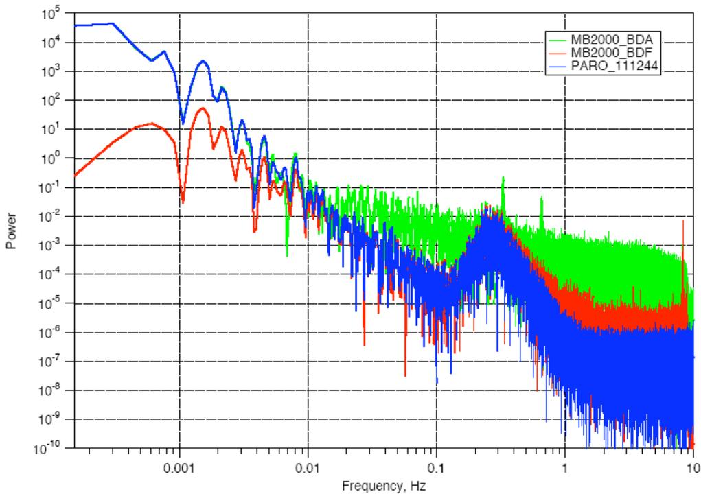
Fig. 10: Spectral comparison of ambient atmospheric background in Pa<sup>2</sup>/Hz. The blue curve is a nano-resolution barometer with a low-pass frequency cutoff at 1.4 Hz. The red curve is the MB2000 with a roll-off at 0.01 Hz. Between 0.01 and 1.4 Hz, both sensors should see the same spectral density, however, the MB2000 appears to be noisier around 1 Hz.
