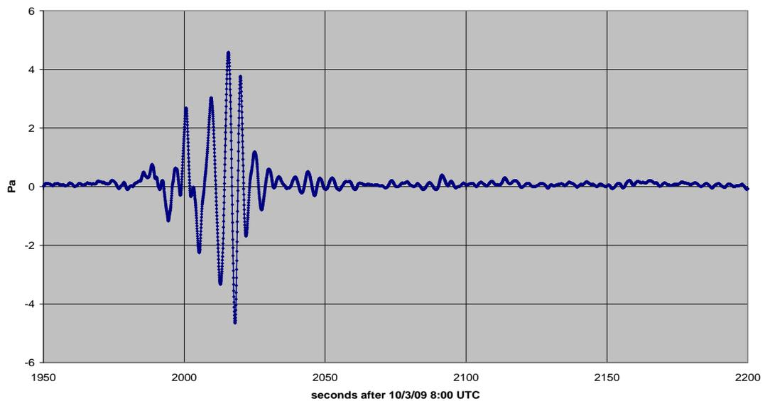
Fig. 5: Detail of Fig. 4. The main shock wave reached the station at 8:33 UTC (48 minutes after the explosion). The wave was dispersed over almost a minute because of different frequency-dependent propagation velocities in the atmosphere, followed by 15 minutes of smaller infrasonic signals. The spacing of data-points (dots) is 50 ms.
