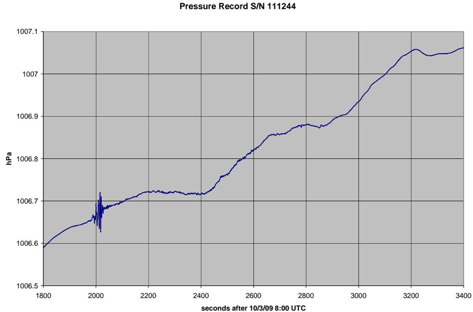
Fig. 3: Pressure recorded for one of two nano-barometers connected to crossed pipes. The recorded pressure is in absolute units of hPa. The volcano signal arrived at 2000 seconds after 8:00 UTC and is visible in the raw pressure record. The atmospheric background signal is very quiet on this particular day.
