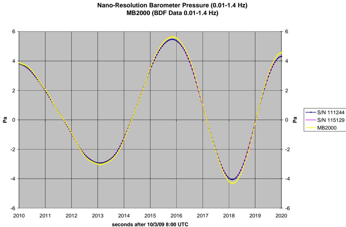
Fig. 8: A comparison of the largest signals recorded after the volcano eruption between two nano-resolution barometers and a micro barometer MB2000. At this scale the nano-resolution barometers track each other perfectly with an NIST traceable scale factor accuracy of 0.01 %. The scale factor of the MB2000 is about 4 % larger.
