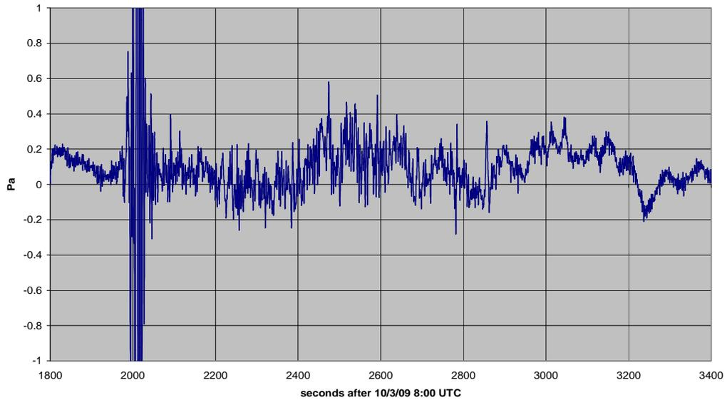
Fig. 4: The pressure data of Fig. 2 high-pass filtered at 0.05 Hz. The infrasound signals from the eruption lasted until 8:50 UTC. Prior to the shock wave and to the far right, the infrasonic background largely consists of microbaroms, generated by standing ocean waves with typical excursions of 0.1 Pa at 0.2 Hz.
