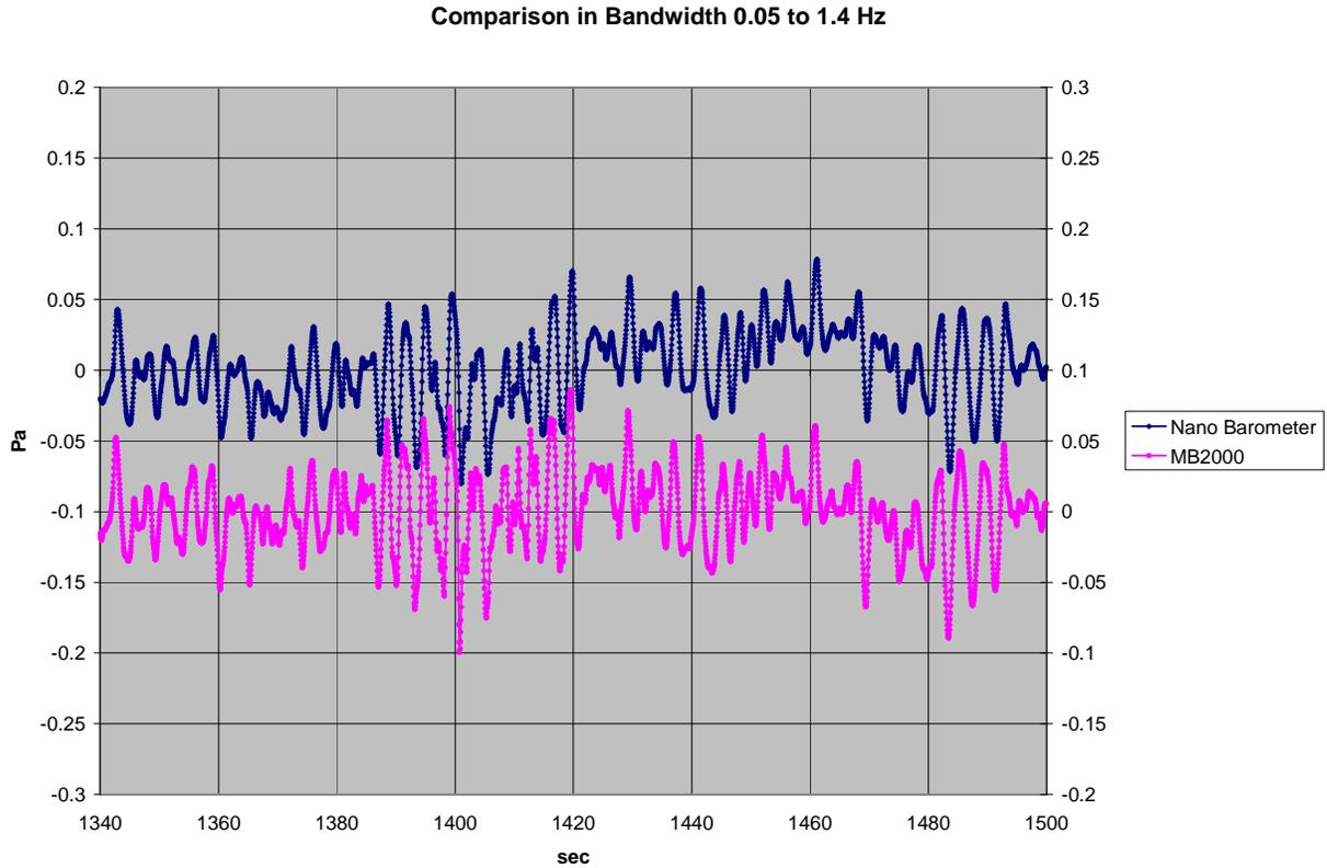
Fig. 9: Typical microbarom background activity measured with a nano-resolution barometer and a micro-barometer MB2000. Both sensors are shown in the bandwidth of 0.05 to 1.4 Hz, but are on different pressure inlets and are pre-filtered differently, so the comparison is not exact. Nevertheless, they track each other well. The comparison of two nano-resolution barometers is shown in Fig. 6.
