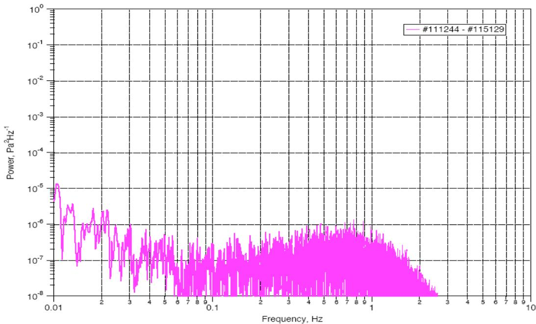
Fig. 7: The uncorrelated noise spectrum between the two nano-resolution barometers provided by the JWA Group. The sensor noise floor spectrum was approximately  $10^{-7}$  Pa<sup>2</sup>/Hz over the infrasound range.
