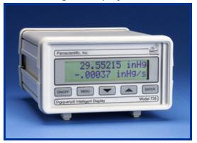
The Model 735 Intelligent Display performs all of the functions of the Model 745 High Accuracy Portable Standard with the frequency inputs from one external Digiquartz® Transducer. It contains an intuitive Front Panel Menu System, Intelligent Interface Board, 2-Line Display, RS-232 communication port, tare capability, and transducer connection terminals.
