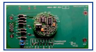
Intelligent Interface Boards are microprocessor-based interface systems that process the frequency outputs from one Digiquartz® Transducer. Dual serial interfaces are available: RS-232 and RS-485. The user may program the sample rate, integration time, engineering units and communication parameters via the serial interfaces. Integrated systems may be formed by combining multiple transducer/board combinations within serial or multi-drop networks.
